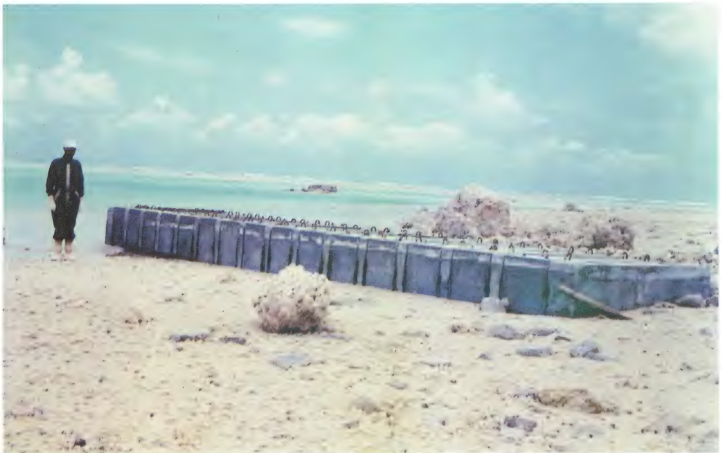
FIGURE 9-16b. HARDTACK, SHOT KOA, ENIWETOK ATOLL, SITE GENE, 13 MAY 1958, 1.37 MT, PHOTO: D + 8, 21 MAY 1958, POST-SHOT CONCRETE BEAM EXP, 6.5 FT. LOWER THAN PRE-SHOT AT 1,830 FT., PO = 1,130 PSI, RA = 2,160 FT.
